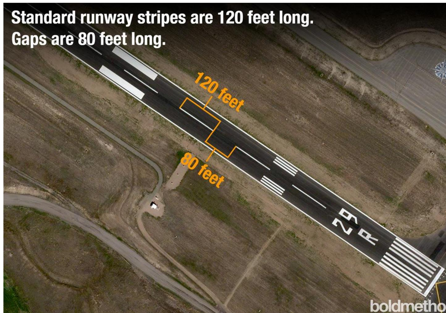
The one major exception to this rule is obvious. Not all runways have perfect stripe lengths. According to the FAA, "Adjustments to the length of the stripes and gaps, where necessary to accommodate the runway length, are made near the runway midpoint." Below are two examples, showing how centerline stripes and gaps are adjusted towards the runway's midpoint.
