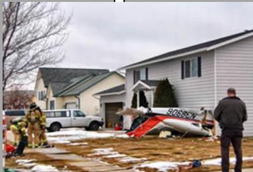
The airplane collided with a number of vehicles and trees, and in the process, the left wing separated from the fuselage. The airplane rotated inverted, and embedded itself into the front of a house. The pilot egressed through the pilot's side window, and he assisted with the egress of his passengers.
