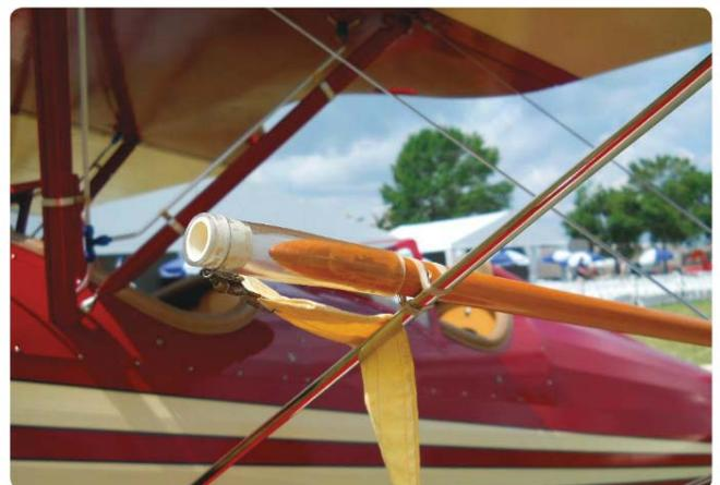
*This owner uses a plastic cap to protect the point of his flying wire stabilizer, with a flag to remind him to remove it before flight.*
